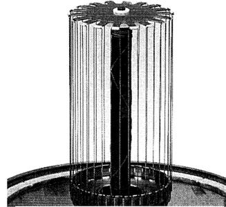
**Figure 5.** Mesh filament structure
