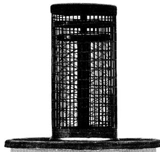
**Figure 2.** Interior assembly of a power tetrode.
