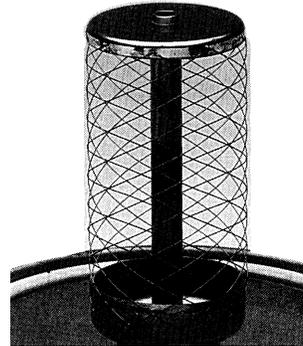
Mesh filaments are composed of filament wires woven to form a basket weave filament structure. (Figure 5.) The wire joints are spotwelded or diffusion bonded at the intersections. Mesh filaments are being designed into most new tube designs on the theory that a mesh filament permits a denser, more closely spaced structure. This allows higher stage gain, increased efficiency and higher frequency operation.
